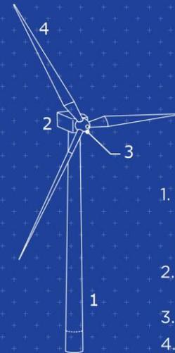
1. Tower (Foundation, Connection to grid, Access ladder, Wind orientation control)
